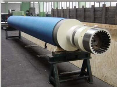
KRAFFT operates as an independent supplier of entire roller systems, i.e. they can be provided including any requested surface plating (e.g. rubber, PU, chrome, etc.) and bearings or similar accessories.
